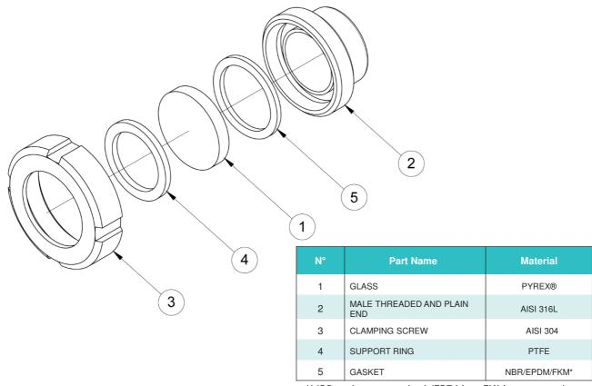
\*NBR gasket as standard (EPDM or FKM on request)
