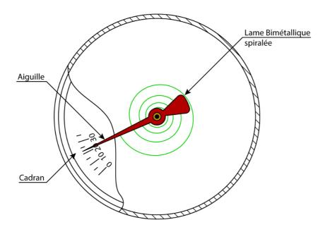
The strip is linked to the needle by a pin. When the bimetallic system distorts, the pin rotates and this rotates the needle.
