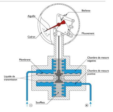
The pressure gauge includes a graduated dial so that the needle points to the measured differential pressure.
