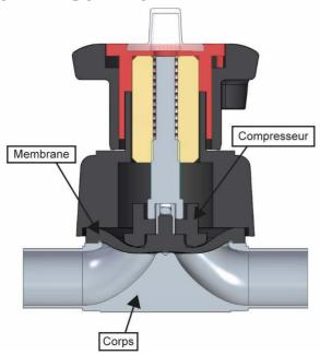
A diaphragm valve is made up of a stainless steel body I, one or several diaphragms 2 and a hand wheel 3 which contains a compressor.
