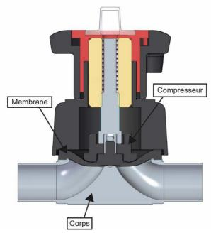
The diaphragm valve is made up of a stainless steel body I, one or several diaphragms 2 and a hand wheel 3 which contains a compressor.
